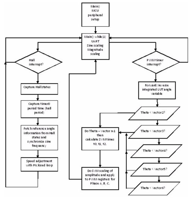
Figure 25. Space Vector Modulation Flow
