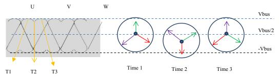
Figure 2. Center Voltage of the Space Vector Floats in Space
