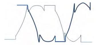
Figure 6. Using  $V_7$  as the Null Vectors in Sector 1, 3, 5 and  $V_0$  in Sector 2, 4, 6
