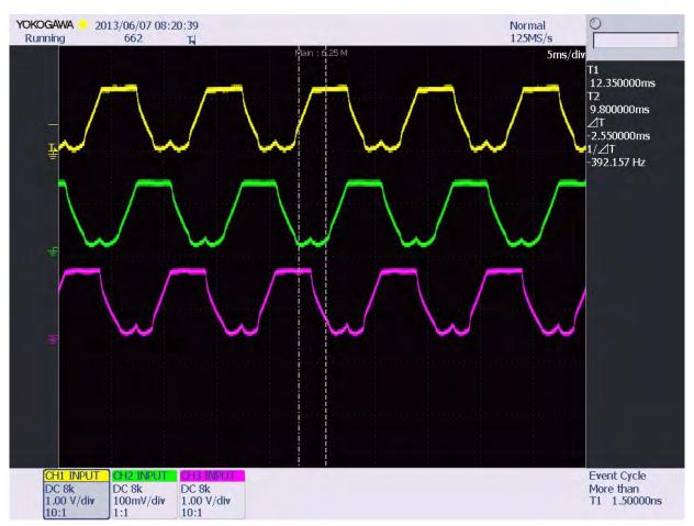
Figure 20. V<sub>7</sub> Zero Vector Only Waveforms
