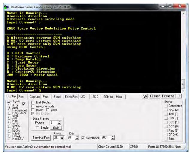
Figure 14. GUI Terminal Showing the " $V_0$ ,  $V_7$  Zero Vector" Switching Pattern
