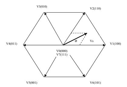
Figure 3. The Rotating Reference Vector  $\mathbf{V}_{REF}$  within the Hexagon
