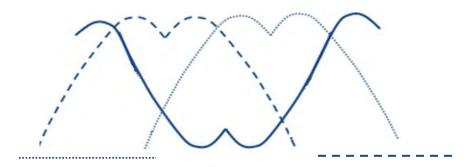
Figure 10. Using Alternate Reverse Switching Modes by Alternating Zeroes for Each Sequence and Reverse Sequence After Each Zero Vector
