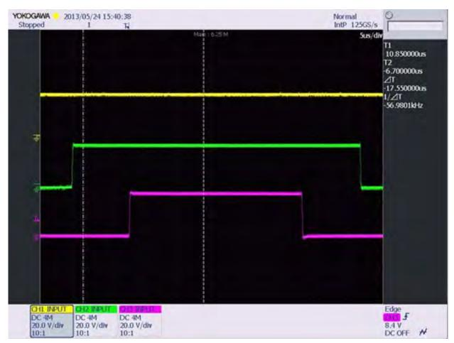
Figure 17. V<sub>7</sub> Zero Vector Only Switching Pattern
