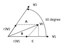
Figure 4. The Location of the Reference Vector in between any of Two Base Vectors
