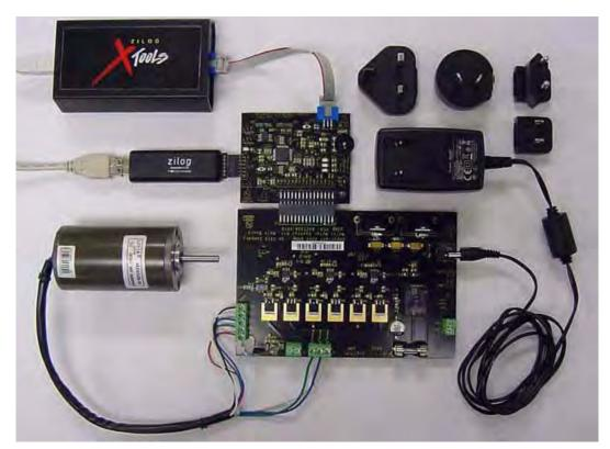
Figure 11. The MultiMotor Development Kit with Z16FMC MCU Module and SmartCable
