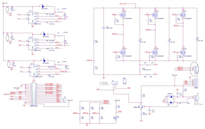
Figure 23. Space Vector Modulation Schematics, #3 of 4
