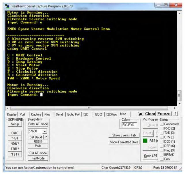
Figure 12. GUI Terminal Showing the Alternate-Reverse Switching Pattern
