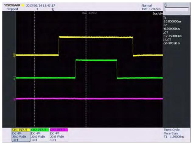
Figure 16. V<sub>0</sub>, V<sub>7</sub> Space Vector Modulation Pattern
