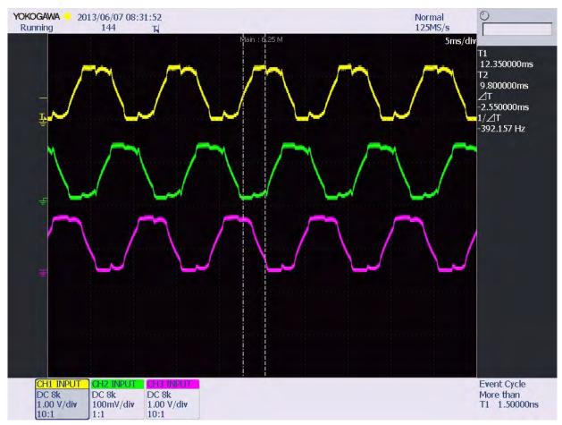
Figure 19. V<sub>0</sub>, V<sub>7</sub> Zero Vector Only Waveforms
